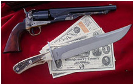
Sheffield pattern blades are not quite as wide as the Black design but most variations carry a false-edged clip point.
